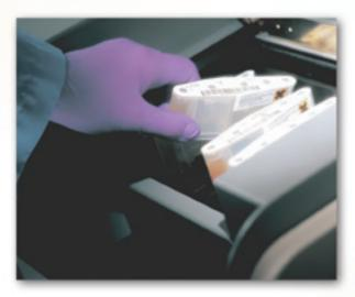
Load any combination of tests - from 50 packs of one assay to one pack of 50 assays - depending on your need.
